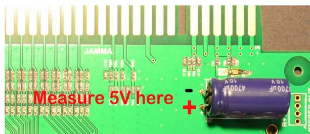
This board operates at 5V. Adjust the voltage as necessary staying below **5.3V absolute maximum**. **Any voltage higher than the absolute maximum will damage PC-JAMMA.**
