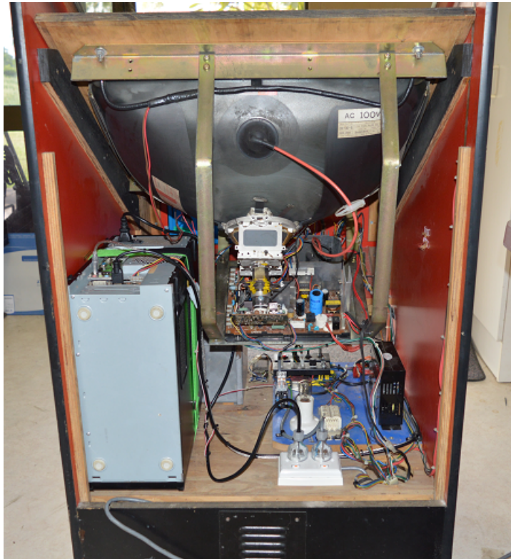
Computer placement in the example cabinet.
