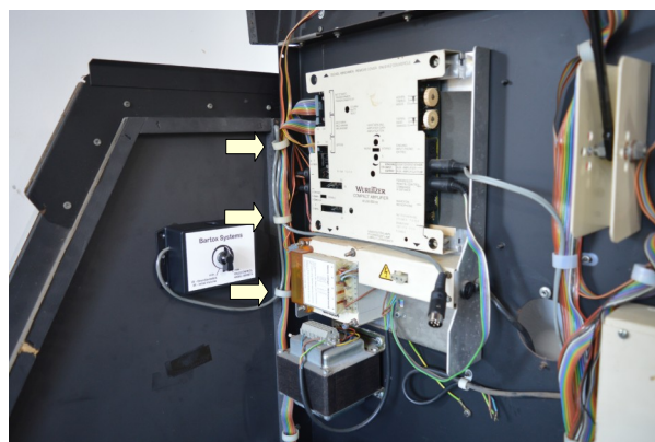
Run the grey cable from the Telecontrol to the amplifier using the cable clamps to neatly secure the excess cable.
