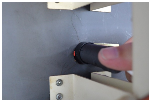
Get the receiver and push it a little way into the P-Clip of the IR mounting bracket.
