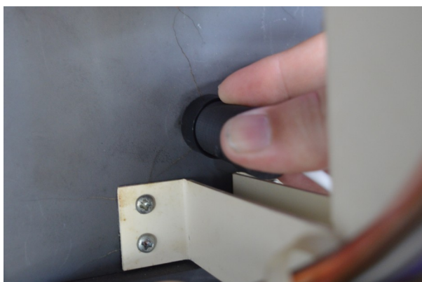
Line up the IR receiver with the hole in the door and push it in the rest of the way. Note that the receiver may need to be pushed in on a slight angle.
