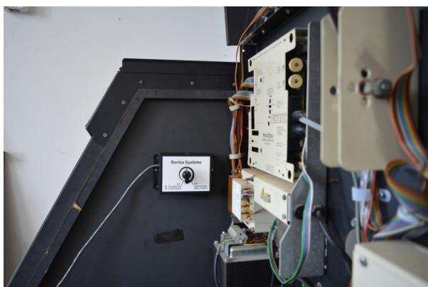
Screw the Telecontrol to the left wall of the cabinet using 46x12mm timber screws or equivalent.
